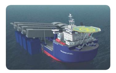
The TML heavy lift system represents a new way of doing marine heavy lift operations. The TML can be used for both removal and installation of platform top sides, jackets, sub sea installations and salvage operations.
