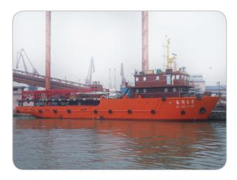
The vessel is made of steel. It adopts transverse framing structure, transom bow and transform stern. There is a two courses deckhouse at the bow and the quarter deck is air rifle operation deck. The vessel has two engines, two fixed pitch propeller and two streamlined hanging rudder. It is applicable to air rifle seismic exploration in shelf area.
