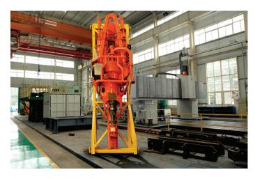
height of mast, and reverse reaming, rotate drilling pipe, circulate mud etc to pass through jamming point to prevent from accidents. Comparing with normal drilling methods, top drive system has incomparable advantages. It has been used for some high challenge and complex wells, such as exploration well, direction well, horizontal well, ERD well, etc, which has been proved to be of great economical interests.
